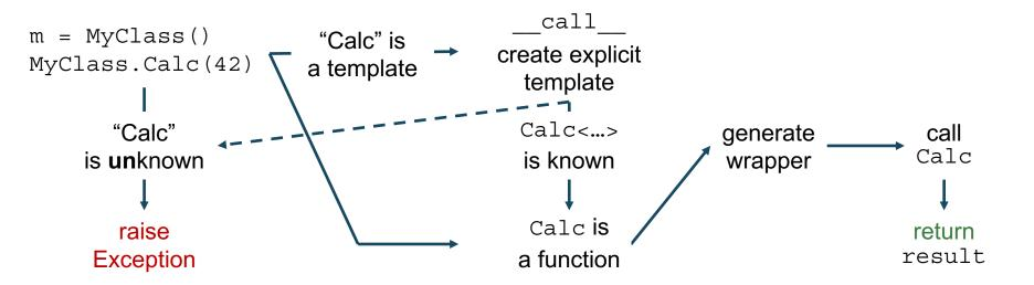
Wrappers of generated (and JITted) C++ are used to easily cover a range of C++isms, such as linkage of inline functions, overloaded operator new, default arguments, operator lookup, etc., etc. For simple cases in PyPy, direct FFI is used, for improved performance.
